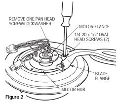
5. Gently snug all flange screws to the motor hub, working around the hub in a clockwise sequence. Next, securely tighten all flange screws, again working in a clockwise sequence. Failure to follow this procedure could result in fan wobble. This completes the blade installation.
